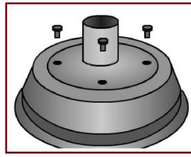
**3.** Bolt the base plate to the base with the bolts provided.
