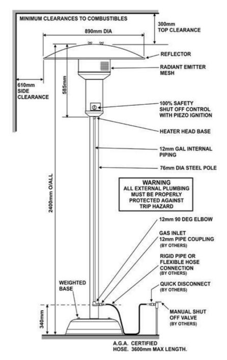
Overall height 2400mm. Overall width 890mm.
