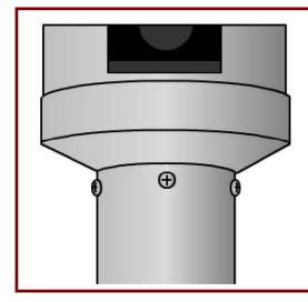
**2.** Fit the pole over the pipe assembly and using the screws supplied fix the pole to the heater head.
