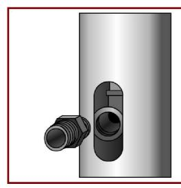
**5.** Fit the hex nipple and socket to the elbow on the bottom of the gas Pipe.
