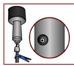
**1.** Screw the pipe and regulator assembly into the heater head. Point the adjustment screw on the regulator to the front of the heater.
