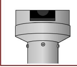
**2.** Fit the pole over the pipe assembly and using the screws supplied fix the pole to the heater head.
