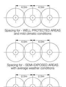
Spacing for - FULLY EXPOSED AREAS with severe weather conditions
