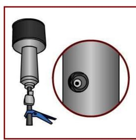
**1.** Screw the pipe and regulator assembly into the heater head. Point the adjustment screw on the regulator to the front of the heater.
