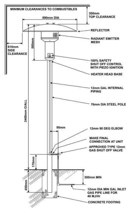
Overall height 2400mm. Overall width 890mm.
